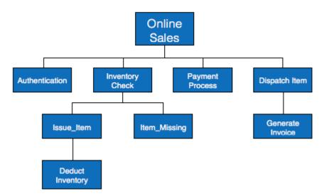
In contrast to IPO (Input Process Output) diagram, which depicts the flow of control and data in a module, HIPO does not provide any information about data flow or control flow.
